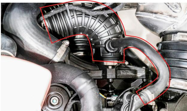
10. Fit the breather filter as pictured using the provided hose clamp.
