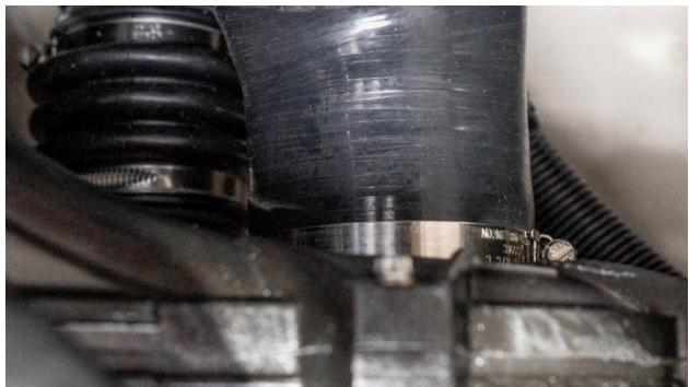
12. Assemble the pod and air filter adaptor with bracket as pictured below. With the pod facing forward, attach the bracket to the left most position on the air filter adaptor.
