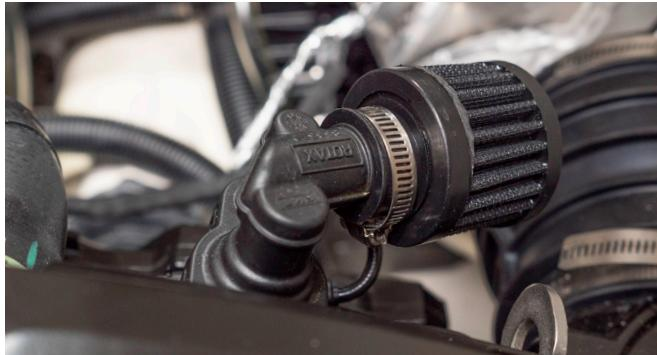
11. Fit the supplied silicon hose to the supercharger using the OEM hose clamp.
